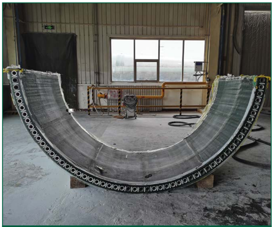
Figure 2. 180 degrees 2.8m pitch circle diameter for 3.XMW, with We4Ce bushings
