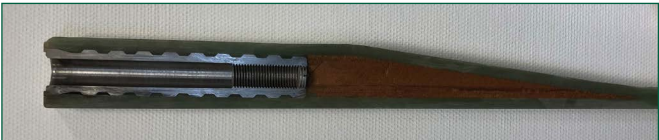
Figure 1. Cross section of the assembled We4Ce bushing solution, post inspection after test
